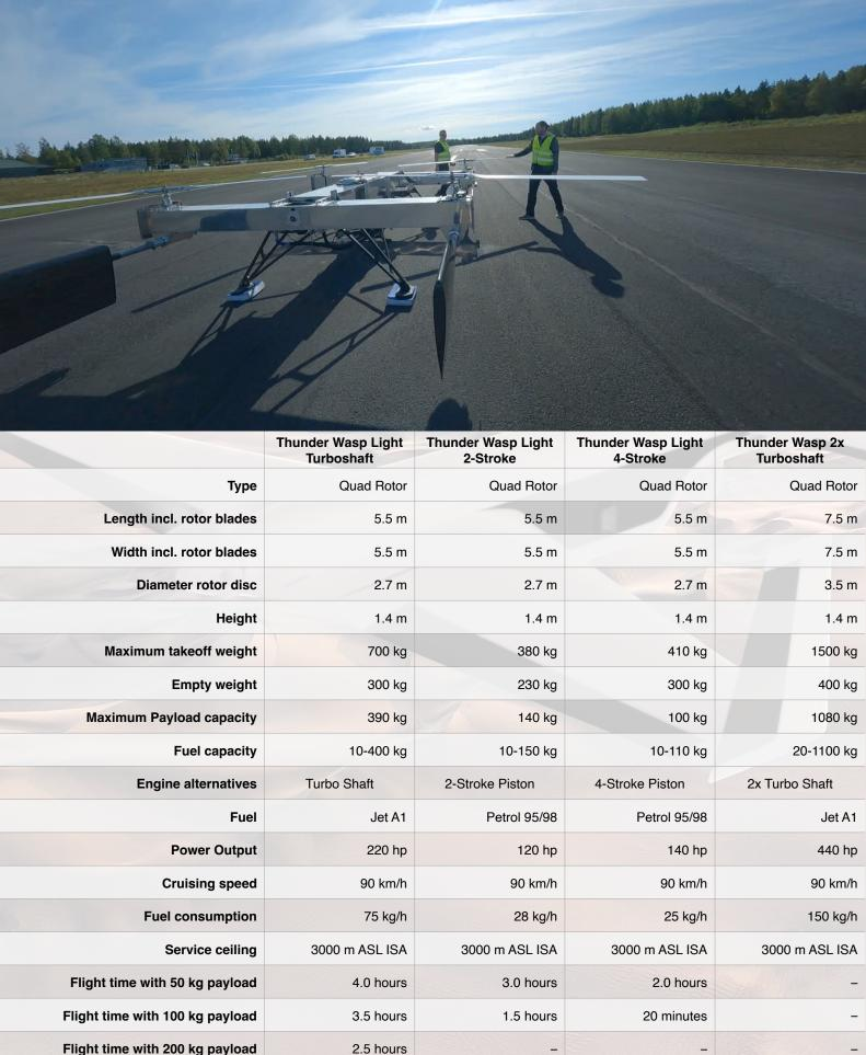
Flight time with 200 kg payload 2.5 hours Flight time with 300 kg payload 1.0 hour Range with 50 kg palyload 360 km 250 km 170 km Range with 100 kg palyload 315 km 120 km 25 km Range with 200 kg payload 200 km Range with 300 kg payload 80 km
